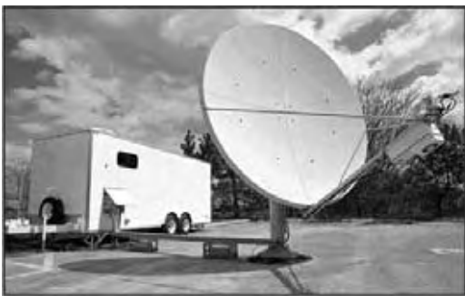
Figure 9.24 Typical 3.4-m hub antenna and 75-cm remote antenna designed for Ka-band service. (Courtesy of NASA Glenn Research Center.)
