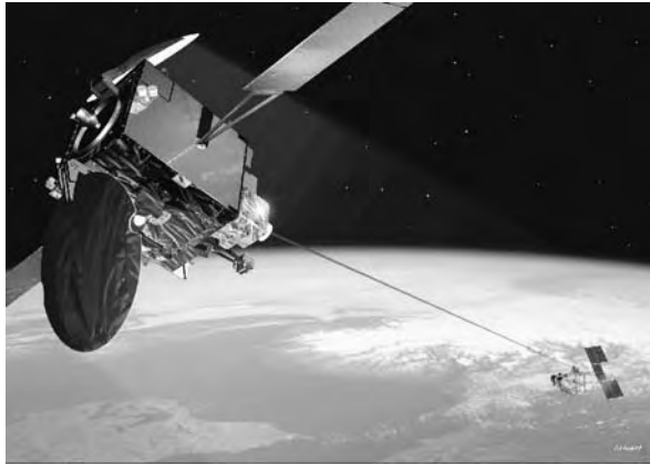
Figure 1.4 Illustration of a laser intersatellite link by the Artemis satellite. (Courtesy of ESTECH.)
