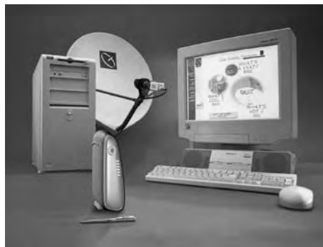
Figure 1.5 Example of a VSAT for broadband communications. (Courtesy of Gilat Satellite Communications.)
