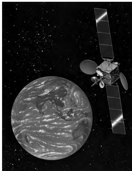
Figure 1.7 AsiaSat 3C is a hybrid C/Ka satellite with a total of 48 transponders.
